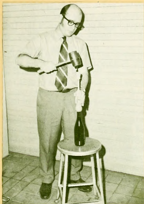
Figure 11. Corking wine bottles with a hand corkscrew which is driven by a mallet.
